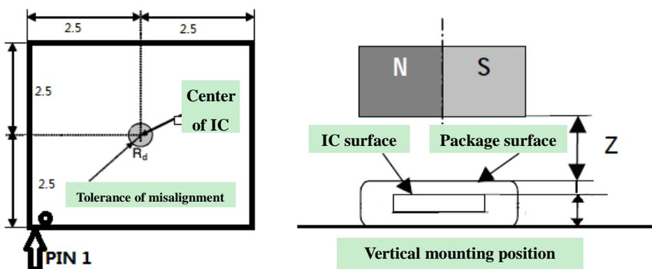
The central axis of the magnet should be aligned with the center of the IC package. The maximum amount of misalignment should be controlled within a perimeter of  $R_d=0.25$ mm. The vertical clearance can be adjusted such that the magnetic field along the IC surface falls between 400 and 900 Gauss. When using the recommended magnet (8mm\*2.5mm), the distance Z is between 1.3mm and 2.5mm.
