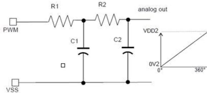
Using large resistance and capacitance values on Rx and Cx shall improve filter performance and ripple rejection, but it may extend the response time of the circuit.
