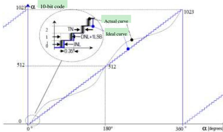
Integral non-linearity (INL) is the maximum difference between the actual position and the measured position.
