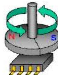
TMR3101 is designed with Tunneling Magnetoresistance (TMR) angle sensors and integrated with digital signal processing circuitry. Paired with a magnet that is magnetized along the radial direction, it can measure 0-360 ° angular position in 10-bit (1024-line) resolution, with the angular resolution at 0.35 °. It supports multiple output interfaces, including PWM, SPI, dual-pulse with zero position, single-pulse with zero position and direction output, or UVW output.
