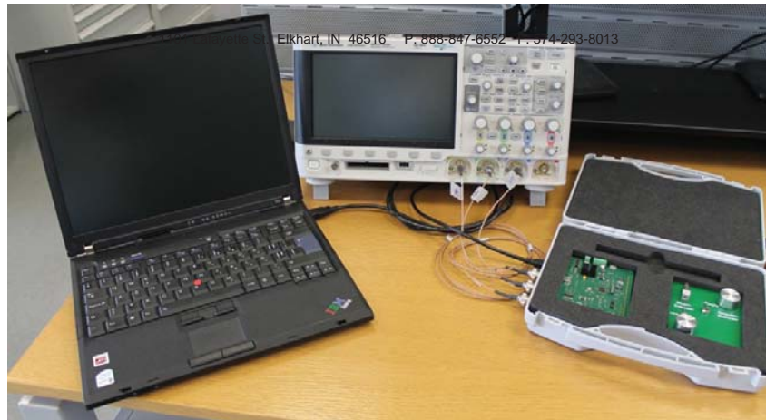
Fig. 9: The signals of the encoder are transferred to the oscilloscope via three coaxial cables
