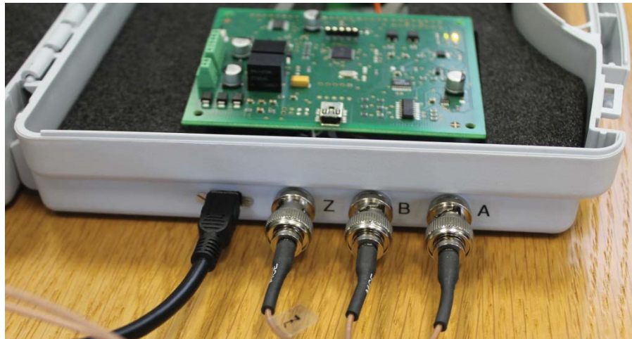
Fig. 8: Demo-Kit connectors for PC (left) and oscilloscope (A, B, Z)
