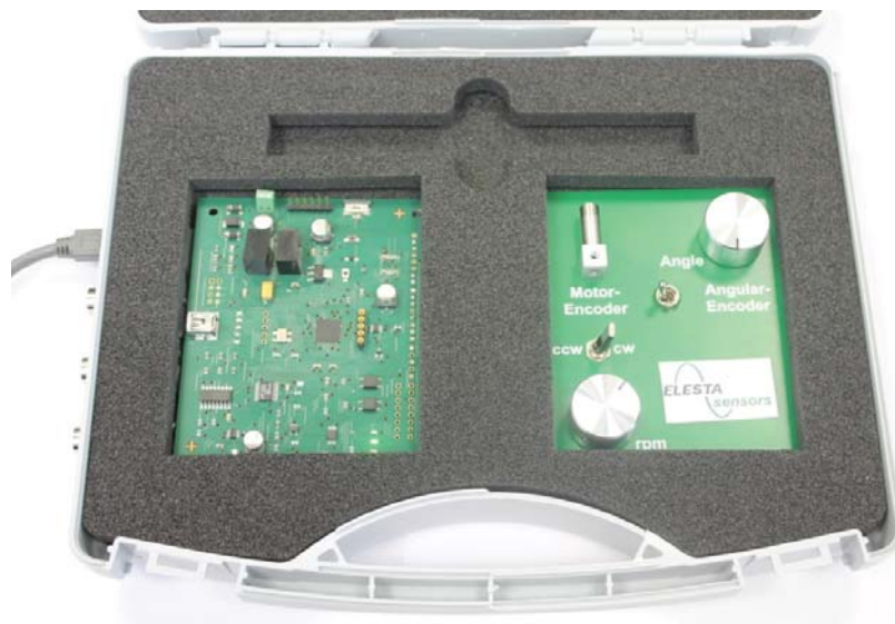
Fig. 7: Demo Case with EFI Board (left) and switching board (right). The USB Type mini B plugged in on the left side.
